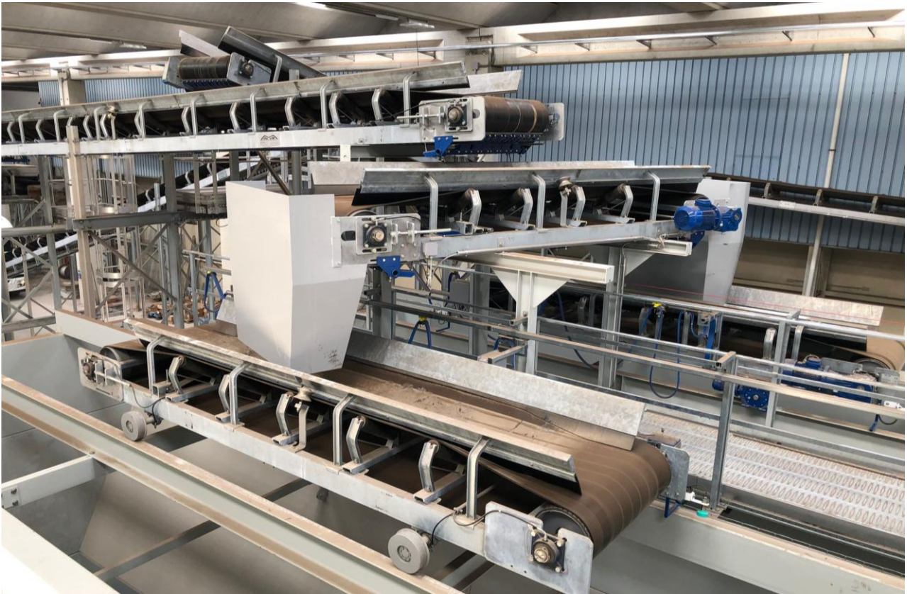
System of diversified mixtures of topsoil and fertilizers
