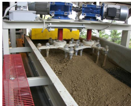
Roller mill feeding system with magnet and double spreading device
