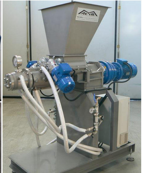
Gypsum extruder with integrated cooling system
