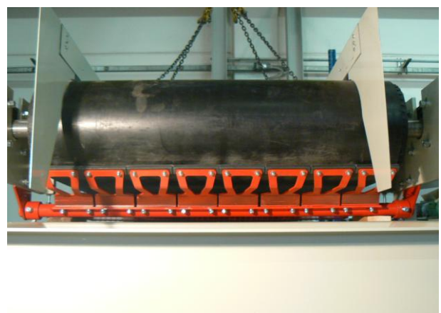
Example of a scraper with pre-loading and with contact points in Widia
