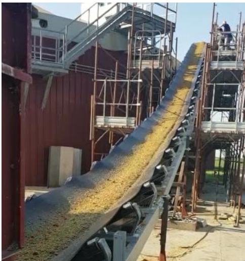
Customized TNV with rubber belts for raw materials feeding in Biogas / Biomethane plants
